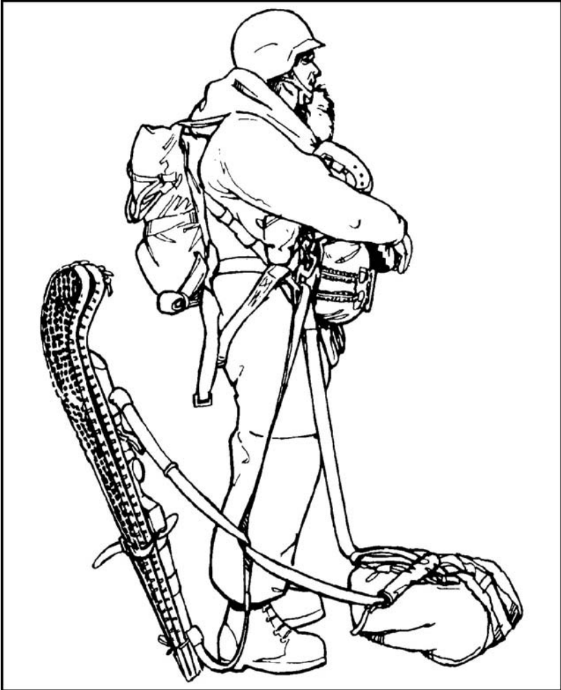
Figure 13-7. Lowering line assembly attached for a tandem load.
